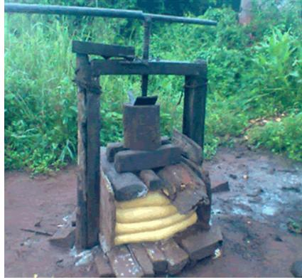
**Figure 1a.** Pressing of grated cassava to release effluent using improved method.
